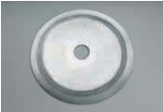
4 Cut the hose by using a proper sharpened disc (see fig. 4), do not use an abrasive disc . The hose must be square and clean cut. Avoid cutting the hose not perpendicularly or cutting the hose causing damages on its wire braid (see fig. 2, 3) for a proper cutting hose operation. Clean the hose carefully from any cutting residue.
