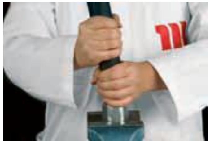
5 Secure in position the socket i.e. by using a bench vice. Screw the hose counter clockwise into the socket until it reaches the bottom. Unscrew 1/4 turn to prevent damage in screwing.
